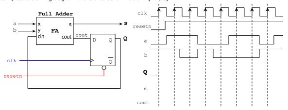
Complete the timing diagram of the circuit shown below: (7 pts)
