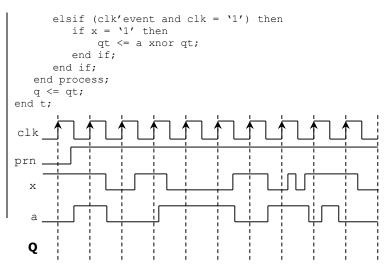
• Complete the timing diagram of the following circuit:  $Q = Q_3Q_2Q_1Q_0$  (10 pts)
