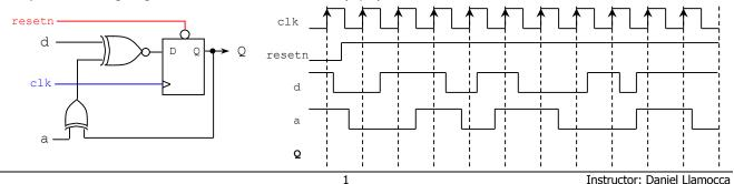
Complete the timing diagram of the circuit whose VHDL description is shown below: (6 pts)
